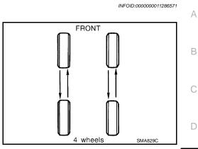
• After tire rotation, perform ID registration. Refer to WT-34, "Work Procedure".
