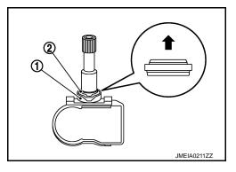
$\bullet$  The cut part A of washer becomes in the center of valve stem.
