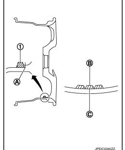
c. If calculated balance weight value exceeds 50 g (1.76 oz), install two balance weight sheets in line with each other as shown in the figure.
