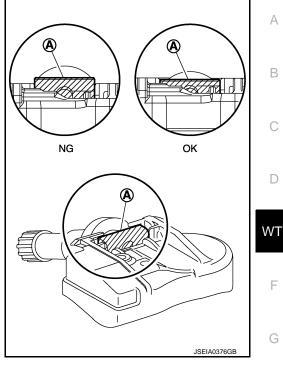
c. Hold tire pressure sensor as shown in the figure, and press the sensor in the direction shown by arrow ((+) to bring it into absolute contact with road wheel. After this, tighten valve nut to the specified torque.
