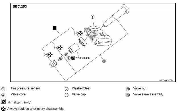
Parts that are replaced as a set when the tire is replaced.
